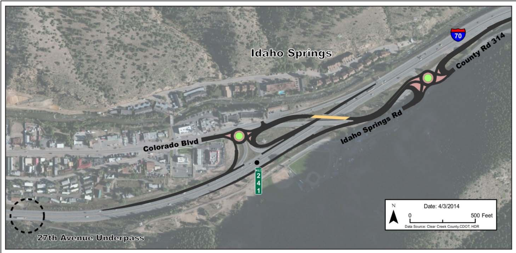
Figure 2-4. Exit 241 Bridge Replacement and Interchange Improvements
