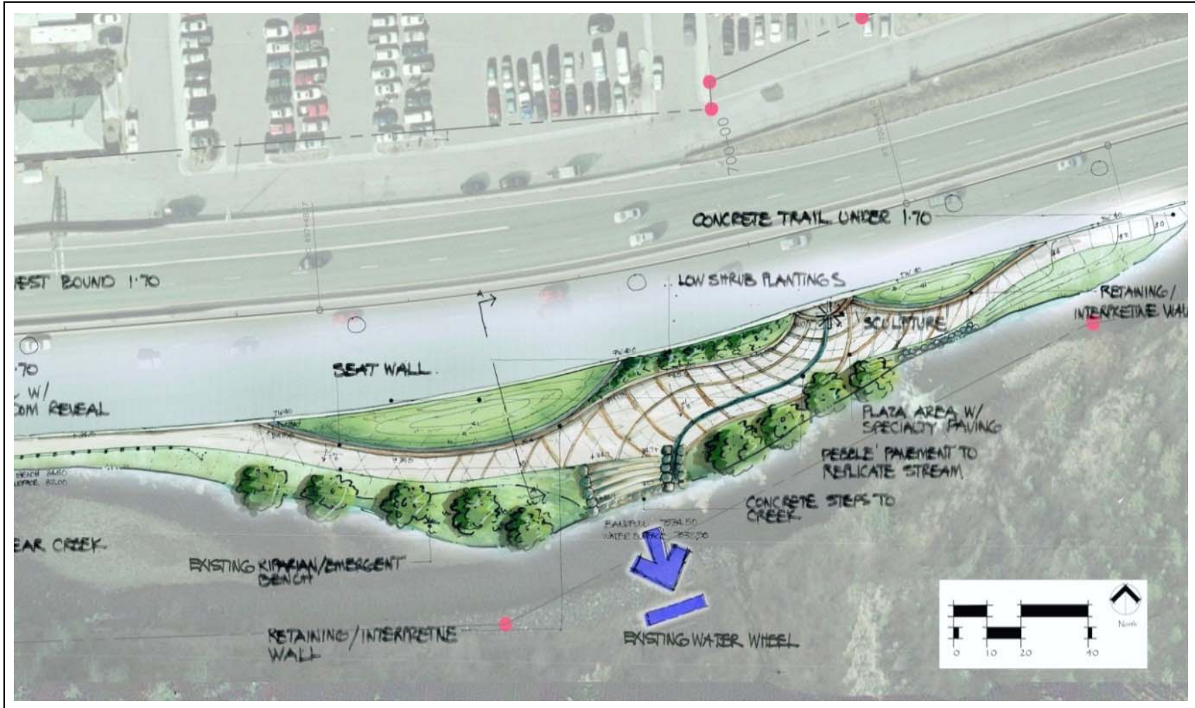
Figure 2-5. Improvements for Water Wheel Park
